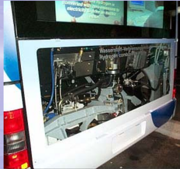
Hydrogen ICE inside a transit bus
