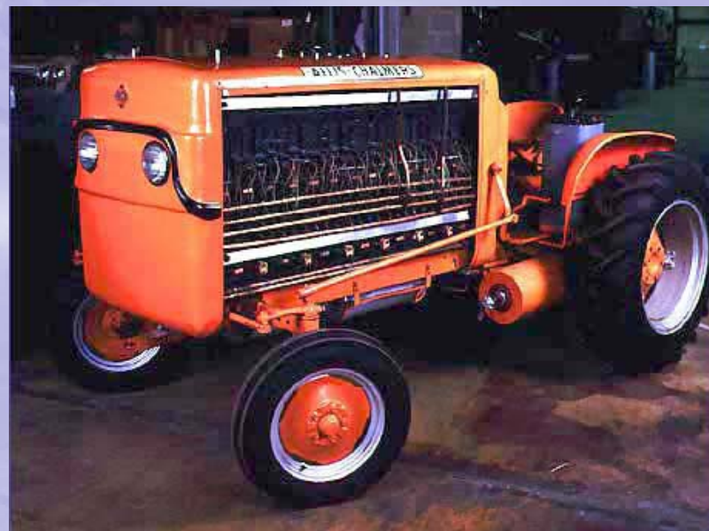
Allis-Chalmers fuel cell tractor, 1959. A year after developing the fuel cell tractor, Allis-Chalmers produced a fuel cell forklift that could lift a 2,000-pound load off of the ground
