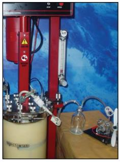
Hydrogen from confectionery waste in a demonstration reactor passes via a glass 'trap' to a fuel cell which produces enough power to drive an electric fan.
