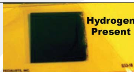
Element One's Thin Film Indicator. The sample decals are coated with the thin film indicator and show the color change when exposed to hydrogen.
